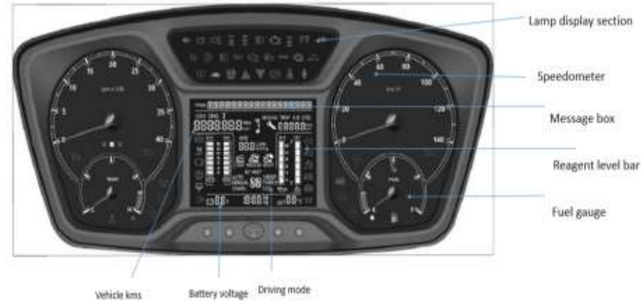
New Multi-Function Ergonomic Instrument Cluster
