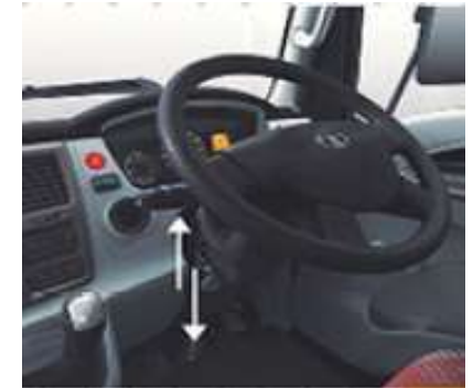
Power Steering with Tilt & Telescopic Feature New Steering Wheel
