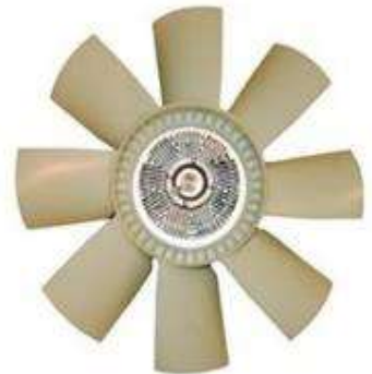
E-Viscous fan to improve the performance of the vehicle
