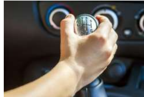
Lower Gear Shift Effort with optimized Gear Shift travel Effort reduced by 30% over BS4
